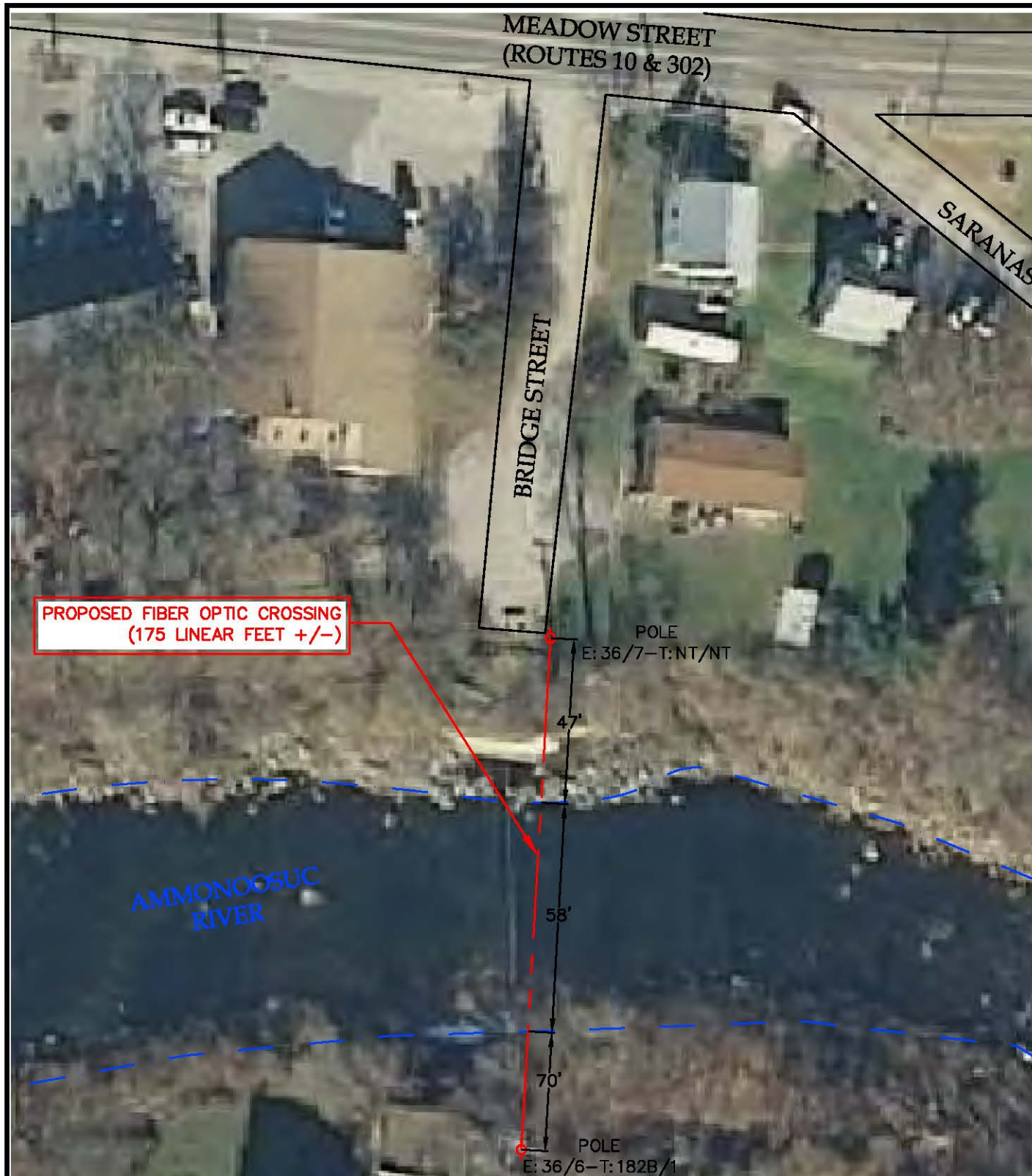
FIBER OPTIC CROSSING - PLAN VIEW WITH AERIAL IMAGE NOT TO SCALE
